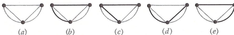
Fig. 3-33: (a) The linear graph of a three-node network. (b), (c), (d), and (e) Four of the eight different trees which may be drawn for this graph are shown by the heavy lines.
