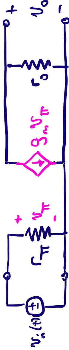
$g_m$  is known as a "transconductance": ratio of current at one place to voltage at another. units are  $\mathcal{V}^{-1}$ .
