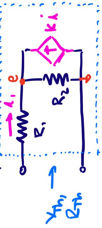
$V_{Th} = \text{"open circuit"} = 0$
