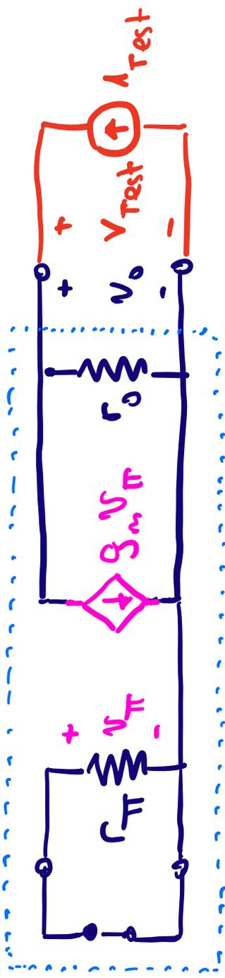
$V_{pi} = 0 \therefore g_m V_{pi} = 0 \therefore V_{Test} = I_{Test} \cdot r_o$
