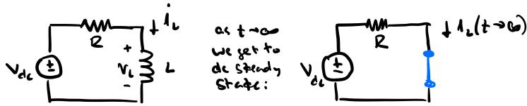
we expect a steady-state solution of 1, (00) = Vac/C. which is exactly what we got from the differential equation! (Likewice, in a capacitor circuit we would replace the capacitor with an open circuit to find the de Steady-State response.)
