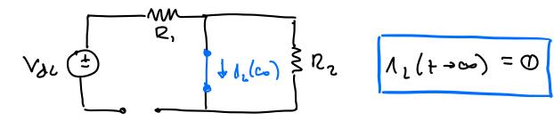
3) The transition from the initial condition C too to the finel value C t= Do must have a time constant of L/RTL
