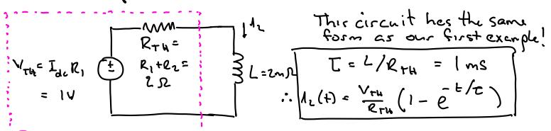
Because we can always reduce the resistor + source network to a Therenin equivalent, we can always solve easity for any 1st order inductor system, we will always get a time constant
