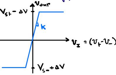
One way we can use an op-amp is as a comparator. (then are special versions designed specifically for use as comparators, though we condo this Function with most op comps).
