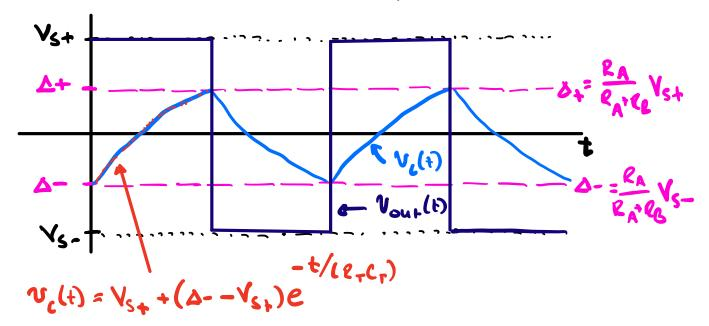
The oscillation period is related to the output saturation voltages (new Vs+, Vs-), hysteresis bend size at - & - (determined by Rea, Re) and the time constant RTCT
