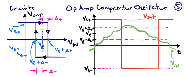
The transition threshold is different for positive - and negative - going transitions, so we also notact chartering at the boundary! (Positive feedback provide hystoris.)
