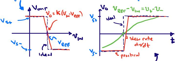
In reality, the speed with which the output can switch is finite, with a limiting "slew rate" in output voltage that depends on the difference between V, V- up to a practical meximum that depends on the device,
