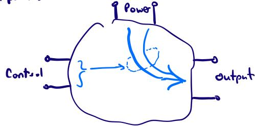
The need for amplification is so common that engineers have developed a class of electronic building blocks that realize this function: The Operational Amplitur, or Op-Amp
