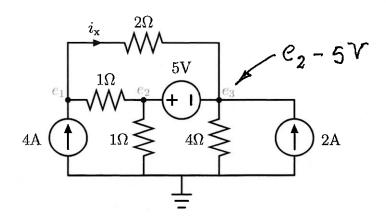
(4A) Write two node equations that can be solved for the unknown node voltages  $e_1$  and  $e_2$ .
