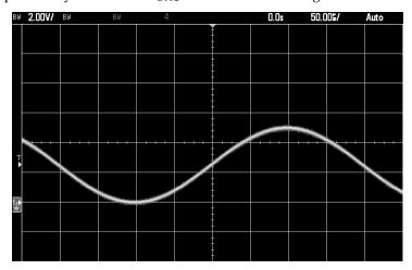
Then, with the scope probes still connected, you hook up a speaker (modeled as a  $4\Omega$  resistor) to the port labeled  $v_{\rm DAC}$  and see the following instead (note that the scales on the scope have been set differently between the two measurements):
