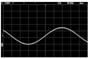
Then, with the scope probes still connected, you hook up a speaker (modeled as a  $4\Omega$  resistor) to the port labeled  $v_{\text{DAC}}$  and see the following instead (note that the scales on the scope have been set differently between the two measurements):
