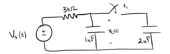
(4A) For all time  $t < t_0$ , assume that  $V_S = 0$  and the switch is open. At  $t_0 = 0s$ , the source steps up to  $V_S = 7V$ . Determine the value of the voltage across the 1uF capacitor after 6 milliseconds,  $v_c(6ms)$ .
