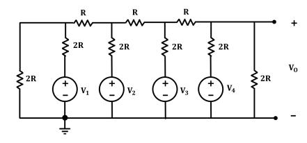
(2C) What is the smallest non-zero voltage, and the largest voltage, that the newly-proposed DAC can produce? Please answer in terms of N, R and  $V_{\rm B}$ .
