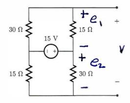
(3B) A 20- $\Omega$  resistor is now connected to the circuit from Part (A) as shown below. What is the Thevenin equivalent of the modified circuit as viewed from the indicated terminals? Numerical results with appropriate are expected.
