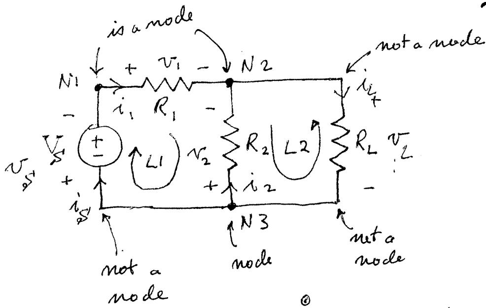
$$\textcircled{2} \quad N1 \Rightarrow i_{s'} - i_1 = 0 \quad N2 \Rightarrow i_1 + i_2 - i_L = 0 \quad \textcircled{3}$$
