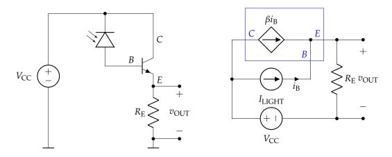
where we have modeled the photodiode as a simple ideal current source whose strength  $I_{\text{LIGHT}}$  is proportional to the light intensity. Our model of the BJT is now contained in the blue box, with the terminals labeled (notice it has been rotated 1/4 turn counterclockwise relative to thee original layout).
