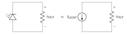
There are a lot of problems with this readout, one being that the readout resistor needs to be quite large to get a substantial voltage, which means circuits that use it will tend to be slow (for reasons we'll discuss in future lectures). To make a fast amplifier, we can use a device called a Bipolar Junction Transistor, which is a three-terminal device and that we are going to model as a linear CCCS.
