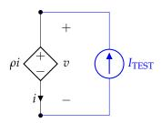
We can analyze this circuit fairly easily by noticing that  $i = I_{\text{TEST}}$  (that is always by construction when using the test source method), and the output  $v = \rho I_{\text{TEST}} = \rho i$ ; thus, the constitutive relation actually is just Ohm's law for a resistance  $\rho$ . From this, we conclude indeed  $V_{\text{TH}} = I_{\text{N}} = 0$ , and  $R_{\text{TH}} = \rho$  so the equivalent circuit is just:
