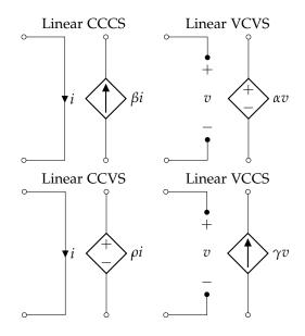
When doing superposition, it is best not to turn off the dependent source. Because the dependent source has a constitutive relation that depends on a branch variable, it is not truly an input to the linear function. If you do turn it off, you'll have to do a nasty backsubstitution step, and it will make a mess of your problem. Better to avoid.
