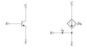
This circuit can be applied directly to the problem of amplifying a photodiode basically by applying the current from the photodiode to the base terminal of the transistor. The result is that instead of  $i_{\rm B}$  traveling through the readout resistor,  $\beta i_{\rm B}$  travels through the readout.
