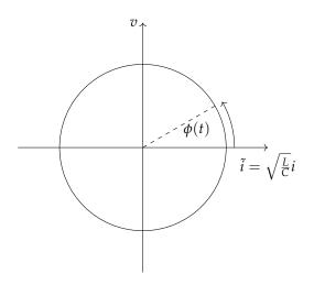
As for the subtleties we observed in the analogous section above, there are a couple changes. First, the oscillatory frequency is no longer simply 1 rad/sec. Because of the transformation of the time variable from *t* to  $\tilde{t} = t/\sqrt{LC}$ , the new radial frequency is  $\omega_{\circ} = 1/\sqrt{LC}$ . Second, the conserved quantity is now proportional to
