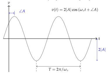
The first takeaway is that the system is oscillatory. Next, observe that it has a **resonant frequency**  $\omega_{\circ} = 1/\sqrt{LC}$  that does not depend on the initial state. Finally, observe it has a phase shift and amplitude that do depend on the initial state.
