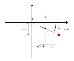
Figure 2: Being able to sketch this construction to quickly identify the sine and cosines of an angle is a good skill to have at hand when dealing with sinusoidal steady state systems. The need comes up again and again.
