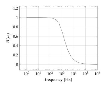
front of cosine ( $H(\omega)$ ) vs. frequency for transfer function where  $\tau = 1 \text{ ms.}$
