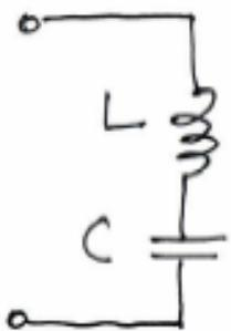
$$Z = j\omega L + \frac{1}{j\omega C} = \frac{1 - \omega^2 LC}{j\omega C}$$
