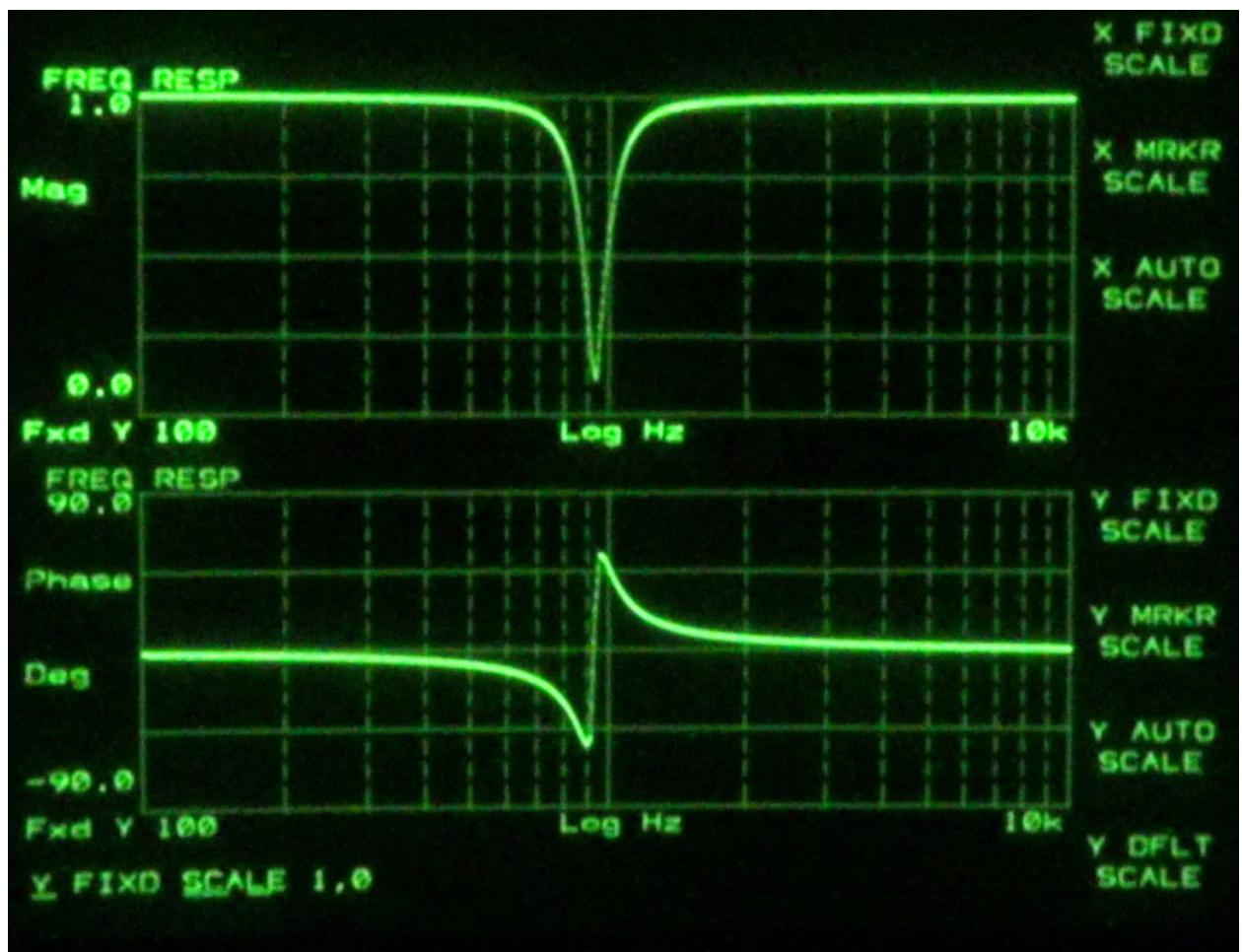
Note that the notch does not go to zero due to the parasitic series resistance of the inductor.
