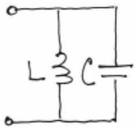
$$Z = \frac{j\omega L \cdot \frac{1}{j\omega C}}{j\omega L + \frac{1}{j\omega C}} = \frac{j\omega L}{1 - \omega^2 LC}$$
