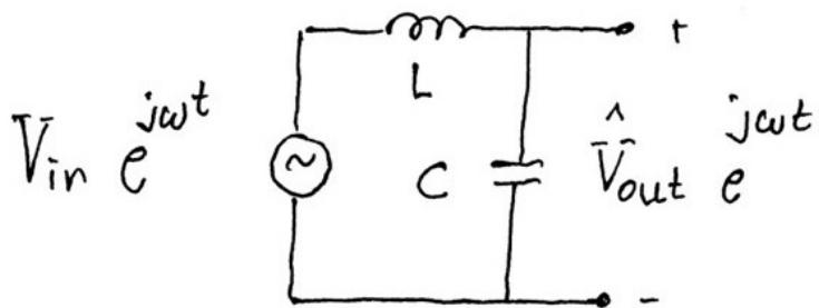
$$\frac{\hat{V}_{out}}{\hat{V}_{in}} = \frac{1/j\omega C}{j\omega L + 1/j\omega C} = \frac{1}{1 - \omega^2 LC}$$
