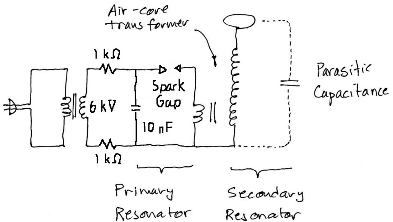
The resistors protect the transformer. At 60 Hz, the transformer fills up the capacitor. When the capacitor voltage gets high enough, the spark gap sparks, and becomes a short allowing the LC resonator to oscillate, driving the rest of the Tesla coil.
