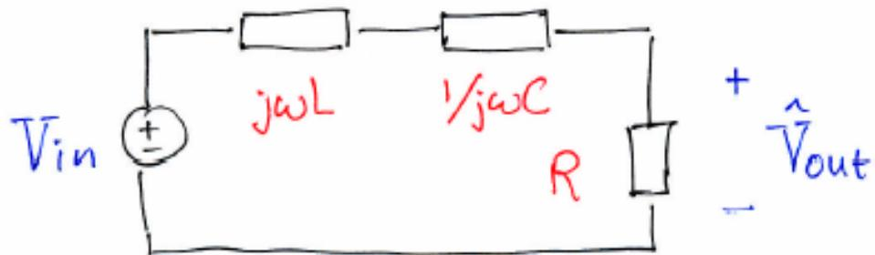
$$\hat{V}_{out} = \frac{R}{R + j\omega L + \frac{1}{j\omega C}} \hat{V}_{in} = \frac{j\omega RC}{1 - \omega^2 LC + j\omega RC} \hat{V}_{in}$$
