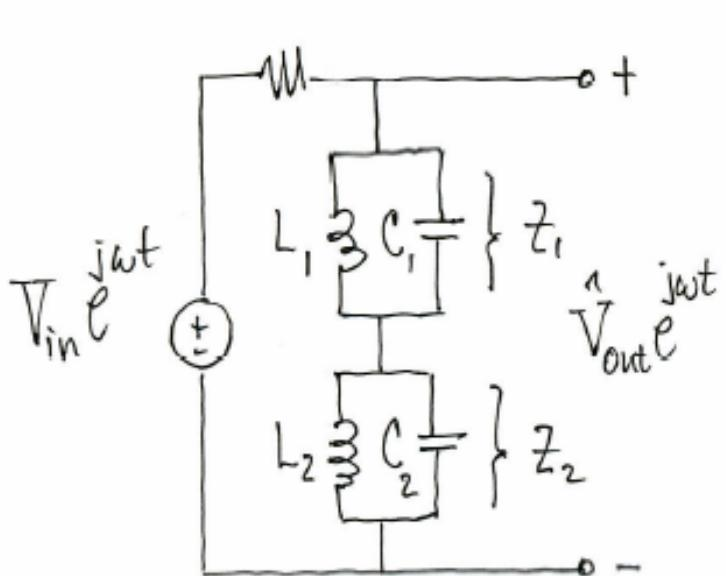
$Z_1 = \text{Open}$  at  $\omega = \frac{1}{\sqrt{L_1 C_1}}$
