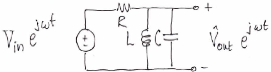
$$\frac{\hat{V}_{out}}{\hat{V}_{in}} = \frac{1/R}{1/R + 1/j\omega L + j\omega C} = \frac{j\omega L/R}{1 - \omega^2 LC + j\omega L/R}$$
