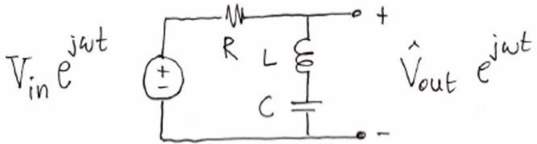
$$\frac{\hat{V}_{\text{out}}}{\hat{V}_{\text{in}}} = \frac{j\omega L + 1/j\omega C}{R + j\omega L + 1/j\omega C} = \frac{1 - \omega^2 LC}{1 - \omega^2 LC + j\omega RC}$$
