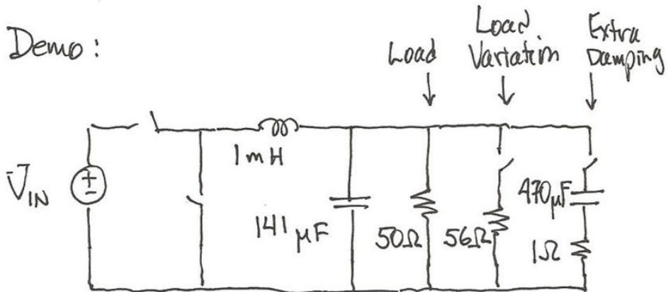
Objective is to reduce the oscillatory load - step response.
