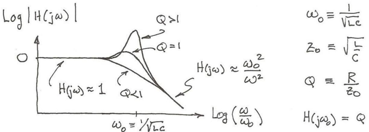
$$\text{Demo} \Rightarrow L = 1 \text{ mH} ; C = 141 \mu\text{F}$$
