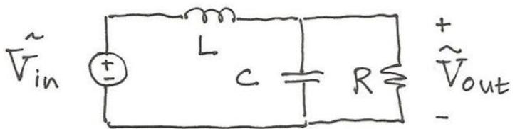
$$\tilde{V}_{\text{out}} = \frac{(R \parallel \frac{1}{j\omega C}) \tilde{V}_{\text{in}}}{j\omega L + (R \parallel \frac{1}{j\omega C})} = \frac{\tilde{V}_{\text{in}}}{1 - \omega^2 LC + \frac{j\omega L}{R}} \equiv H(j\omega) \tilde{V}_{\text{in}}$$
