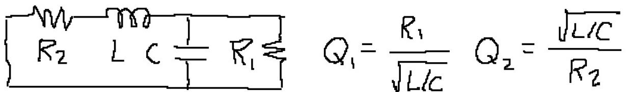
$$L = 1 \text{ mH} \quad C = 141 \mu\text{H} \quad R_1 = 50 \Omega \quad R_2 = 0.5 \Omega$$
