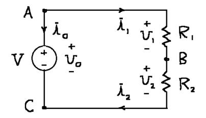
$\frac{Solution}{i_{1} = i_{2} = -i_{0} = V/(R_{1}+R_{2}) = i$   $v_{0} = V ; v_{1} = R_{1}i = V \frac{R_{1}}{R_{1}+R_{2}} ; v_{2} = R_{2}i = V \frac{R_{2}}{R_{1}+R_{2}}$ Note:  $v_{0} = v_{1}+v_{2} = \lambda(R_{1}+R_{2}) \Rightarrow \frac{v_{0}}{i} = \frac{R_{1}+R_{2}}{E#fective R}$
