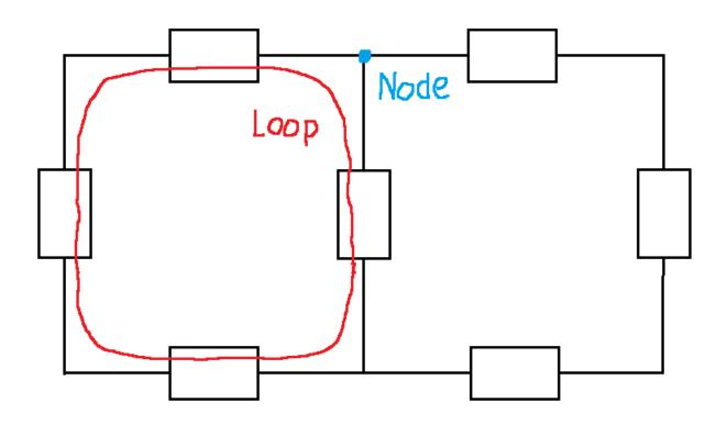
KVL: ∑び=0 Around - Either Loop Direction
