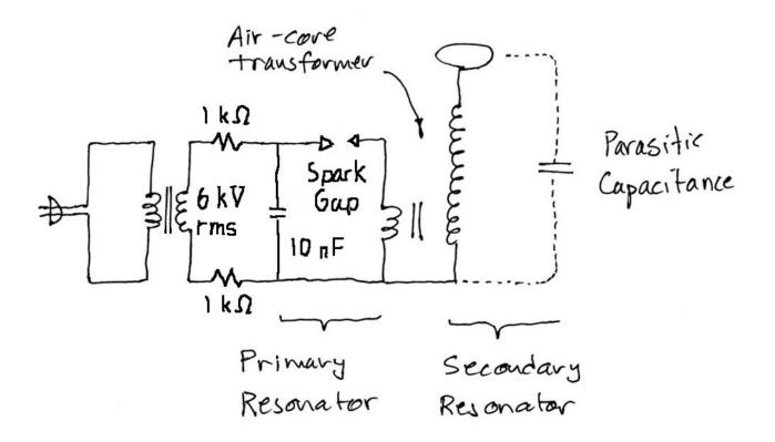
The resistors protect the transformer, which charges the capacitor (+/-) at 120 Hz. When the capacitor voltage gets high enough, the spark gap sparks, and becomes a short allowing the LC resonator to oscillate, driving the rest of the Tesla coil.
