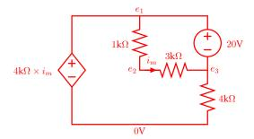
We can start by noticing that the 20V source is connected to two resistors in series (4k $\Omega$  total resistance), so  $i_m = 5 \text{mA}$ .
