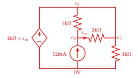
Here, the  $1k\Omega$  and  $3k\Omega$  resistors are in parallel; they form a current divider, so  $i_m = \frac{1}{4}(12\text{mA}) = 3\text{mA}$ .
