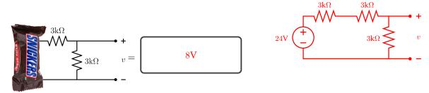
Here we have a voltage divider again, but we have to be careful since we're only measuring the drop across the bottom  $3k\Omega$  resistor; so this voltage divider cuts our Thévenin voltage by a factor of 3.
