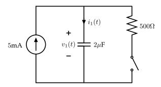
The switch is closed for all time t < 0, such that by time 0 it is operating in a steady state.
