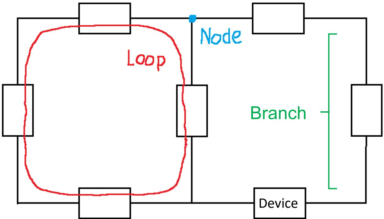
**Device:** a multi-terminal lumped-parameter piece of electrical hardware having identifiable voltages across (between) its terminals and currents through its terminals. Most devices in 6.200 have only two terminals.
