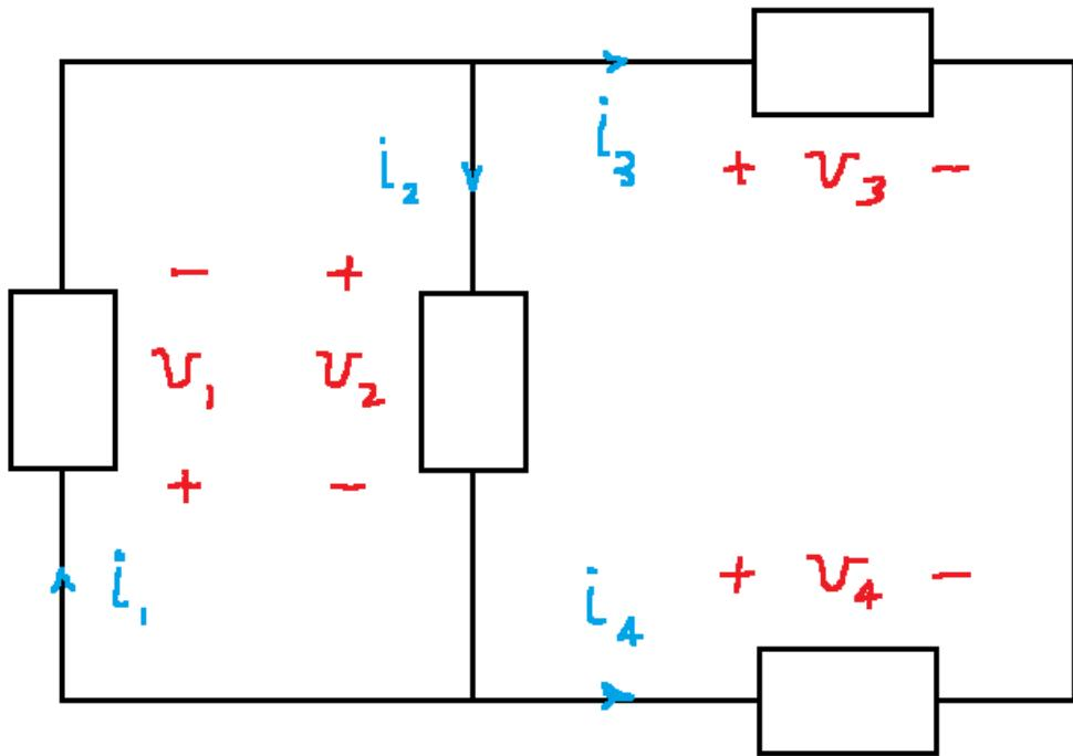
$$KVL: -V_1 - V_2 = 0 \quad \text{or} \quad V_1 = -V_2$$
