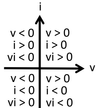
Tellegen's Theorem states that any circuit, linear or nonlinear, that obeys both KCL and KVL conserves energy and power at all times such that  $\sum_n v_n i_n = 0$  where  $n$  indexes the devices in the circuit.
