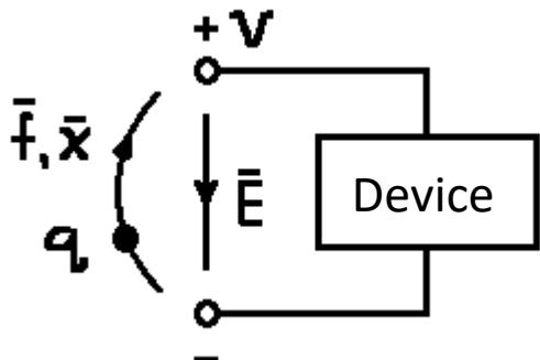
Lifting charge  $q$  across the terminals of the device requires energy  $W$
